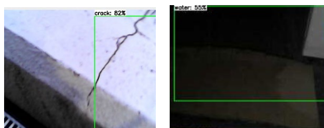
(a) Crack recognition by the robot (b) Water recognition by the robot Fig. 9. Object detection result.
