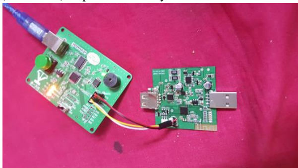
Fig. 3. Programming the device with Nordic Semiconductor Development Kit
