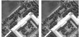
Figure 8a – Original Image. Figure 8b – recovered image from 20% of original data (1.6 bits per pixel, SD = 6.2).
